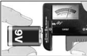
Connect the 9V Battery
